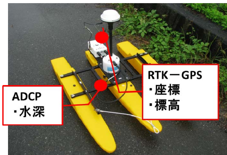
図-7 観測機材 (ADCPとRTK-GPS)
